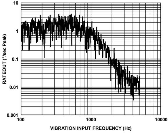
Figure 16. Typical Response to 10 g RMS Sinusoidal Vibration
