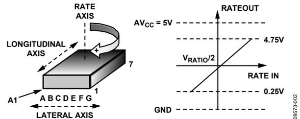
Figure 2. RATEOUT Signal Increases with Clockwise Rotation
