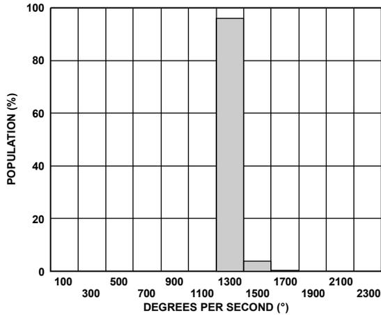
Figure 10. ST2 Output Change at 25°C ( $V_{RATIO} = 5 V$ )
