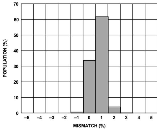
Figure 11. Self-Test Mismatch at 25°C ( $V_{RATIO} = 5 V$ )
